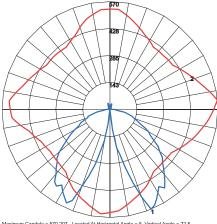
Maximum Candela = 570,207 Located At Horizontal Angle = 5, Vertical Angle = 22.5 # 1 - Vertical Plane Through Horizontal Angles (5 - 185) (Through Max. Cd.) # 2 - Horizontal Cone Through Vertical Angle (22.5) (Through Max. Cd.)
