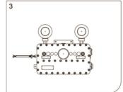
Install pipe to 3/4 NPT entry and fix 16mm (0.63inch) Chico A.
