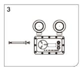
Install pipe to 3/4 NPT entry and fix 19mm (0.75inch) Chico A.
