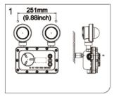
Drill two holes as fig. 1, the distance as per 251mm (9.88inch).
