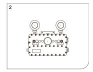
Fix with four 5/16-inch expansion screws.
