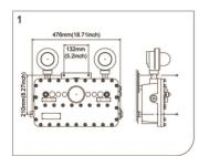
Drill two holes as fig. 1, the distance as per 476mm (18.74inch) and 132mm (5.19inch).
