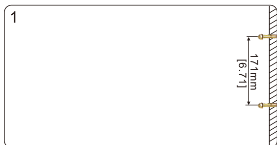
1. Drill 2x Ø15 hole for expanded screws, and fix them to the wall. (Horizontal distance: 171mm)
