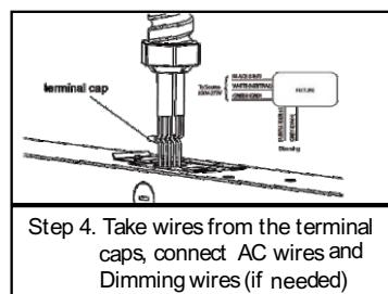
Step 4. Take wires from the terminal caps, connect AC wires and Dimming wires (if needed)
