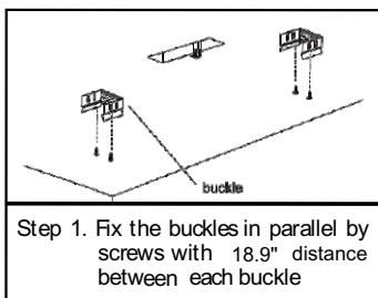
Step 1. Fix the buckles in parallel by screws with 18.9" distance between each buckle
