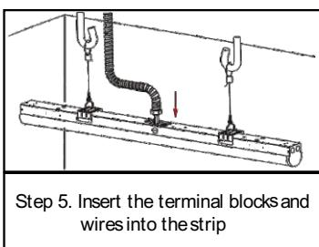
Step 5. Insert the terminal blocks and wires into the strip
