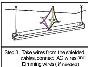
Step 3. Take wires from the shielded cables, connect AC wires and Dimming wires (if needed)
