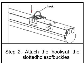
Step 2. Attach the hooks at the slotted holes of buckles
