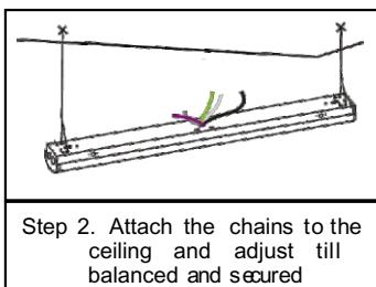
Step 2. Attach the chains to the ceiling and adjust till balanced and secured
