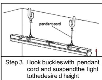
Step 3. Hook buckles with pendant cord and suspend the light to the desired height
