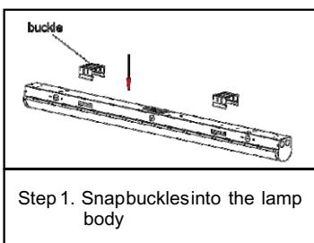
Step 1. Snap buckles into the lamp body
