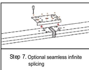
Step 7. Optional seamless infinite splicing
