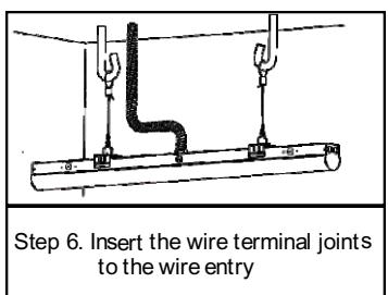
Step 6. Insert the wire terminal joints to the wire entry
