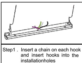
Step 1. Insert a chain on each hook and insert hooks into the installation holes
