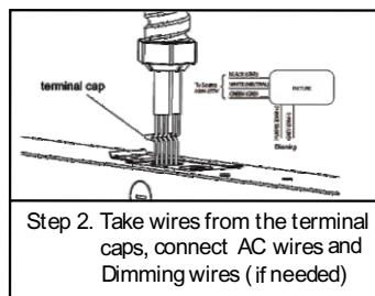
Step 2. Take wires from the terminal caps, connect AC wires and Dimming wires (if needed)
