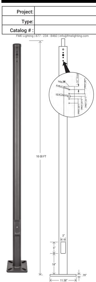
The JMC Series Straight Round Steel poles are built from high strength steel tube and are available side drilled for arm mounted area lighting luminaires or with tenon mounts for flood and post top luminaires. Typical area lighting applications include retail centers, industrial parks, schools and universities, public transit and airports, office buildings and medical facilities. Mounting heights of 10 to 30 feet can be used based on selected luminaire application.
