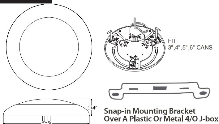
**Snap-in Mounting Bracket Over A Plastic Or Metal 4/O J-box**
